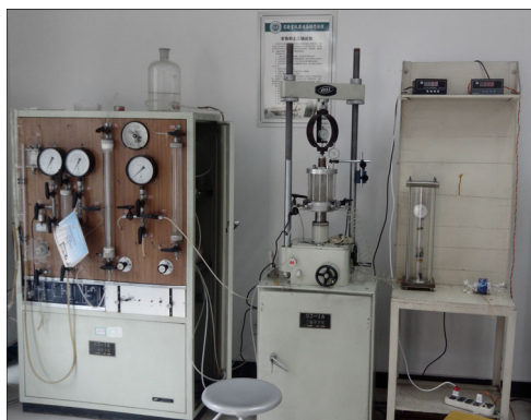
Fig. 2 Triaxial test system of unsaturated soil
