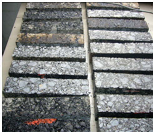
Fig. 2 Small beam specimens of asphalt mixture
