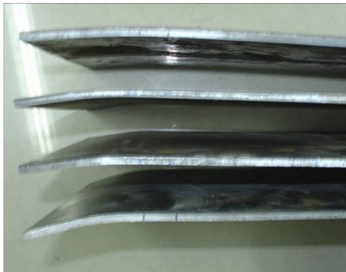
Fig. 3 Crimping parts in experiment (Comparison of crimping parts with different die displacement: h_1=8.32 mm, h_2=9.318 mm, h_3=10.03 mm and h_4=13.95 mm)
